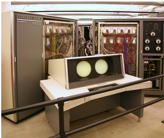
While working at Control Data Corporation in the 1960s, Cray designed the CDC 6600. It is considered the first supercomputer and was the fastest computer in the world from 1964-1969. Image courtesy Jitze Couperus (Flickr).
